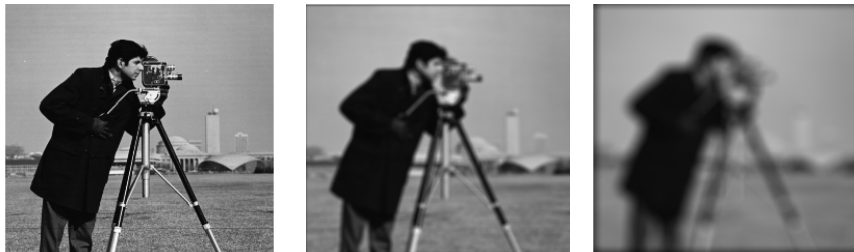
Figure 1. Cameraman image: Pillbox filter blurring achieved at filter radius 3 and radius 9. The first type of blurring is achieved by the use of a circular pillbox averaging filter the more the radius of the filter, the greater the blur. Figure 1 illustrates this.
