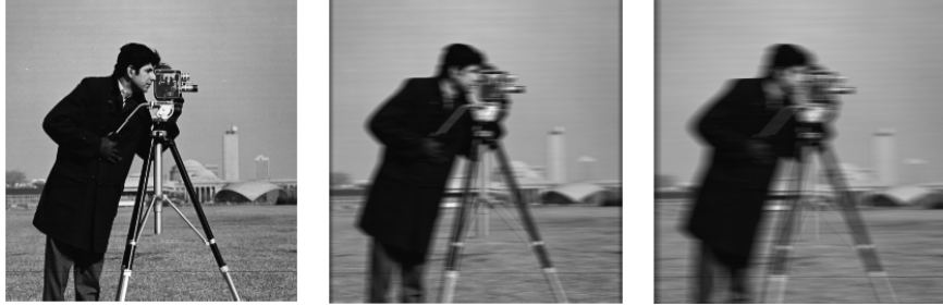
Figure 2. Cameraman image: Motion filter blurring achieved at length 9 and length 15.
